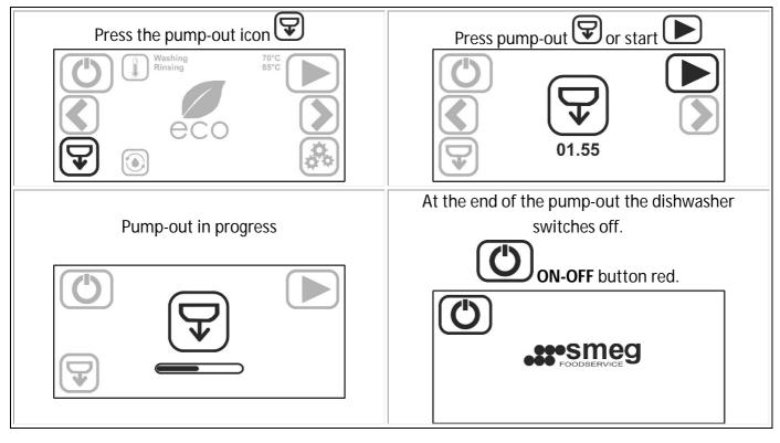
Never switch the dishwasher off with water in the tank; always pump out first. At the end of the working day, after pump-out, the filters should be cleaned.
