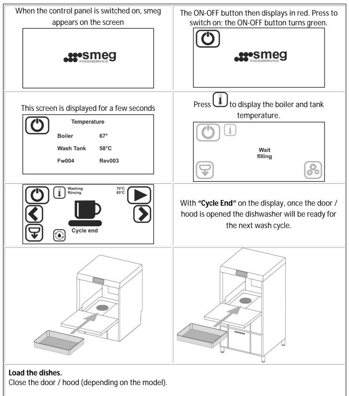
**N.B.:** if the autostart function is set as **ON** and the dishwasher is ready, the cycle starts when the door is closed/the hood is lowered
