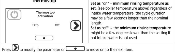
If the thermostop device is set "off" the rinsing temperature are no longer monitored and the user is responsible for ensuring that the minimum correct temperature are maintained for the tank and boiler. It is particularly important to check the intake water temperature. Also refer to the insufficient washing/drying /foam in tank point of the "troubleshooting" section : restore **thermostop ON** and/or connect the appliance to a hot water supply.
