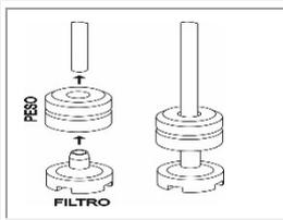
Before inserting the hoses into the containers, fit the weights (needed to ensure that they always draw in liquid from the bottoms of the containers) and the filters onto their ends as shown. If the detergent dispenser is not factory-fitted, it can be retrofitted after ordering the relative kit.
