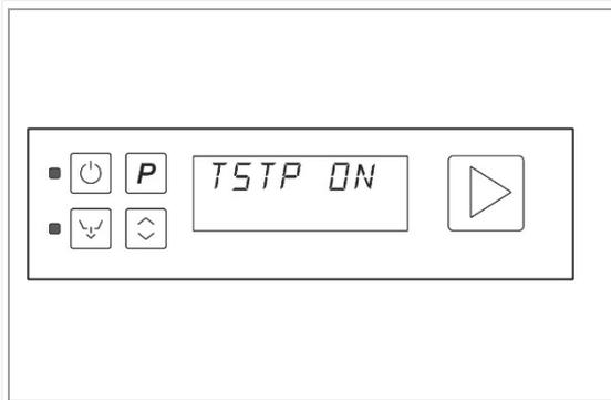
**Set to "on"** = minimum washing and rinsing temperature set for the tank and boiler regardless of the inlet water temperature; the nominal duration of the cycle could be a few seconds longer.
