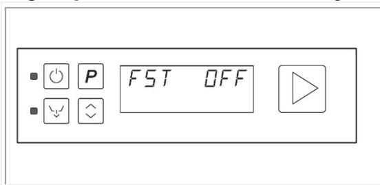
**Fast start (FST):** starts the dishwasher in less than the standard time; leads to higher water consumption for the first cycle start.
