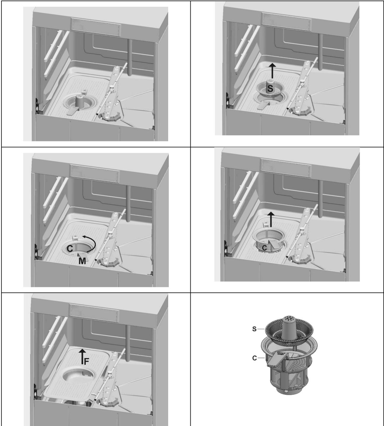
Remove the filters (simply lift them out as shown here), taking care that no large residues fall into the sump underneath. Clean them to remove residues and rinse with plenty of water, then put them correctly back in place; do not use sharp or pointed tools.
