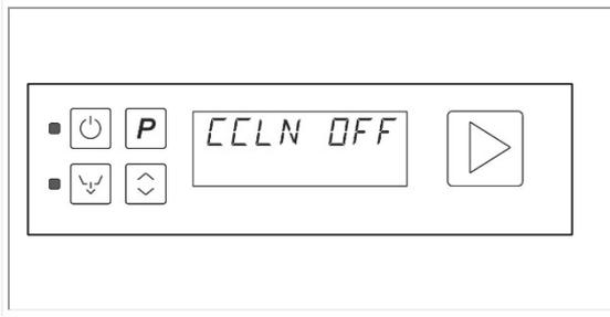
When this option is activated, the appliance pumps out all the water from the tank and then refills it with clean water at every wash cycle. How long this operation takes depends on the washing water temperature.
